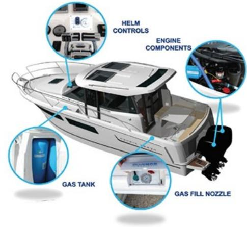
Figure 3 | Propulsion System Based On The LPG Engine
